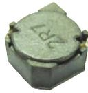
The new **DM5028/DM5048 shielded SMD** power inductor series are developed specially for use as choke in DC/DC converters. For lower DCR and higher saturation current the core material MnZn was selected. The top down constructions features tight tolerance and best solderability.
