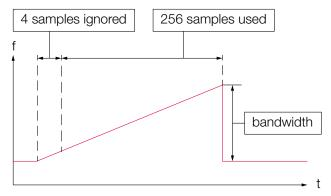
Figure 6: Ramp generation and sampling
