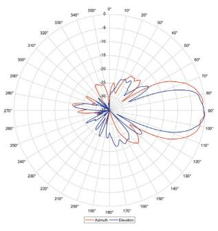
Figure 2: TX relative antenna pattern
