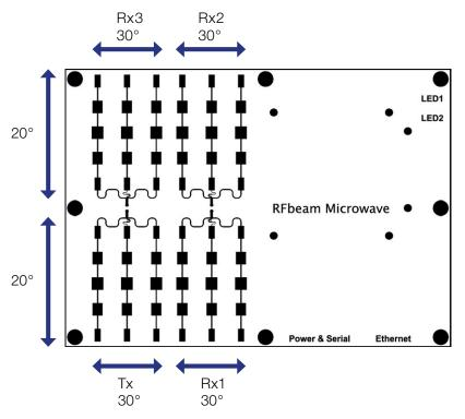
Figure 3: Beamwidth and antenna order
