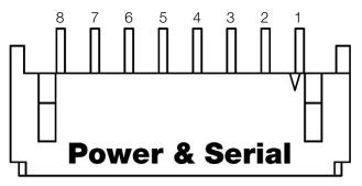
Figure 5: Power and serial connector
