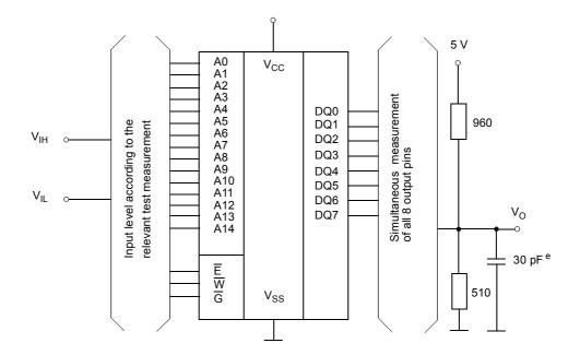
$^{e} \text{ In measurement of } t_{\text{dis}(E),} \ t_{\text{dis}(G)}, \ t_{\text{en}(E)}, \ t_{\text{en}(W)}, \ t_{\text{en}(G)} \ \text{the capacitance is 5 pF.}$
