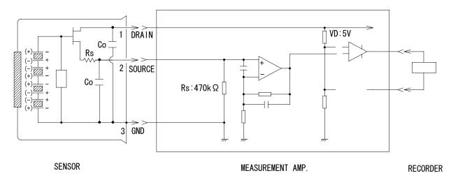
※ Measurement Amp.: Non-inverted type, gain 72.5 dB at 1 Hz , 0.4 to 2.7 Hz
