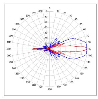
Azimuth 7°, Elevation 25° At IF output voltage -6dB (corresponds to -3dB Tx power)
