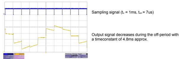
Fig. 8: x\_AC output amplitude decreases during sleep time.
