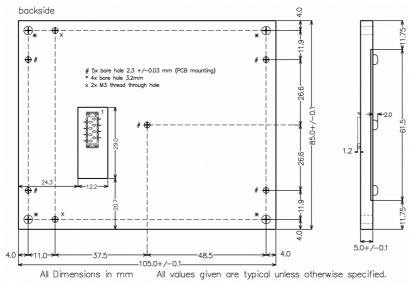
Fig. 4: Mechanical dimensions
