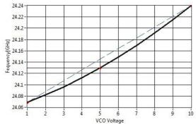
Fig. 3: Typical Frequency vs. VCO voltage
